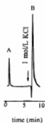
Figure 4. Chromatogram of pepsin and lysozyme in dye bonded PSDVB/PVA microbeads
